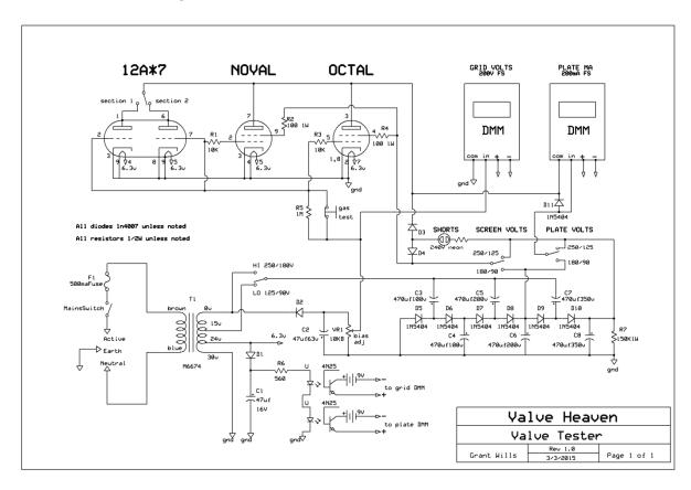
As you can see, the tester is quite straightforward with a 30V 2A transformer doing most of the work. It drives a 4X or 6X voltage multiplier via a "HI/LO" switch to generate 90, 125, 180 and 250 volts for supplying the test voltages for the valve under test. The HI/LO switch feeds the voltage multiplier from either the full 30V from the transformer or from the 15V tap to halve the output voltages.
